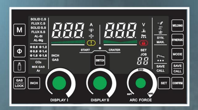
**Digital Display LED Screen:** Display current, voltage, wire-feed speed, parameter reference number, error code and other relevant information.
